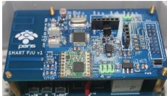
Gambar 5. Modular Hardware Smart PJU
